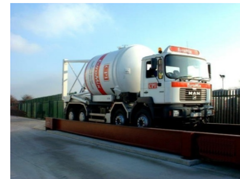
A typical Weighbridge Installation
