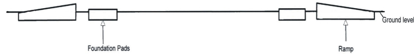
Side view of simple Titan Foundation
